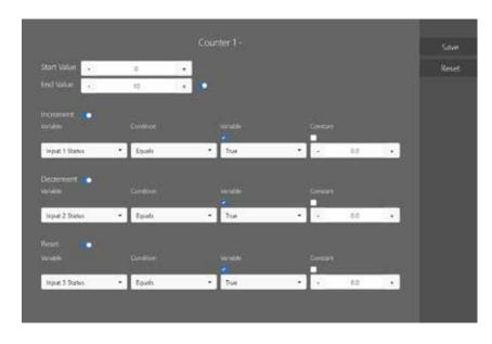
function lines. Depending on which condition evaluates to True, the counter will increment, decrement or reset itself. The PDM counters can count between a value of -2147483647 and +2147483647.
