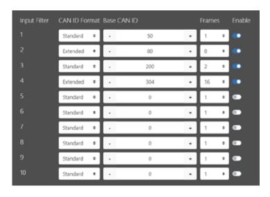
ID onwards, and press enable. It is important to select the correct ID format, consult the instruction manual of the device which is sending the CAN frame to determine which ID is used. Up to 16 consecutive ID CAN frames can be extracted with each filter. Here is a typical example of how the CAN filters may be set up to filter out a range of CAN frames. It is important to note that the IDs are set in decimal format, not hexadecimal.
